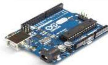
Gambar 1. Papan Arduino Uno R3
